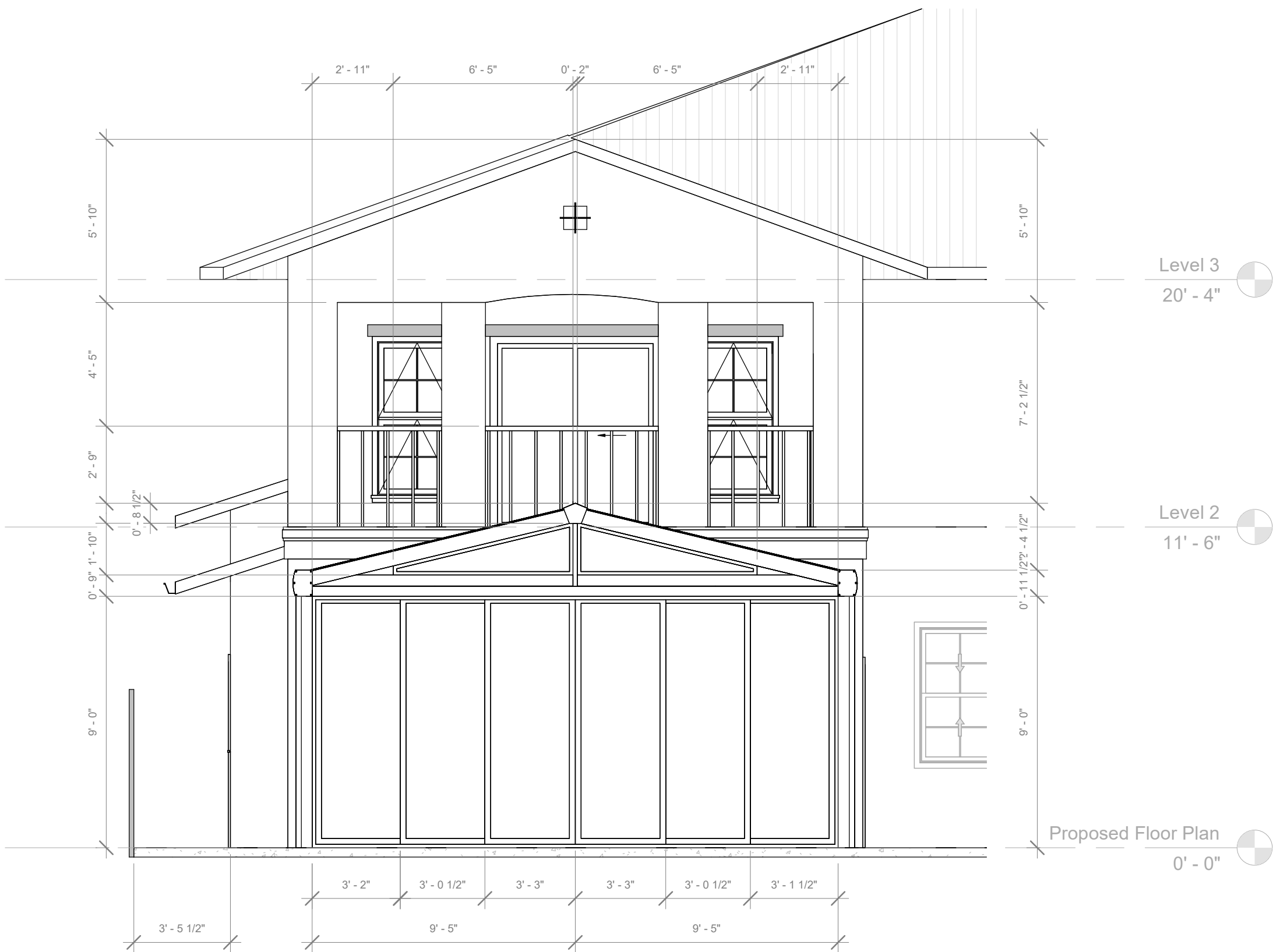
3 Proposed North Elevation with Patio Enclosure 1/4" = 1'-0"
